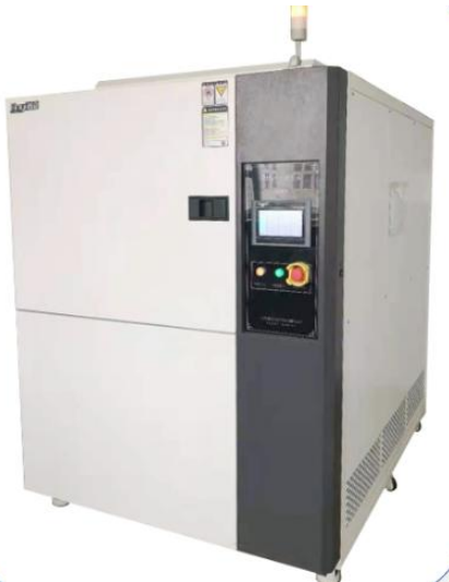
20 L constant temperature and humidity test chamber
