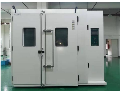
3.6 m3 constant temperature humidity laboratory
